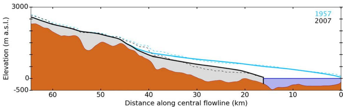
**Fig. 4.** Columbia Glacier main centerline: perfect plastic model profiles ( $\tau_y = 150$  kPa, solid curves) with 1957 and 2007 observations (dashed curves). Note 5:1 vertical exaggeration in scale.
