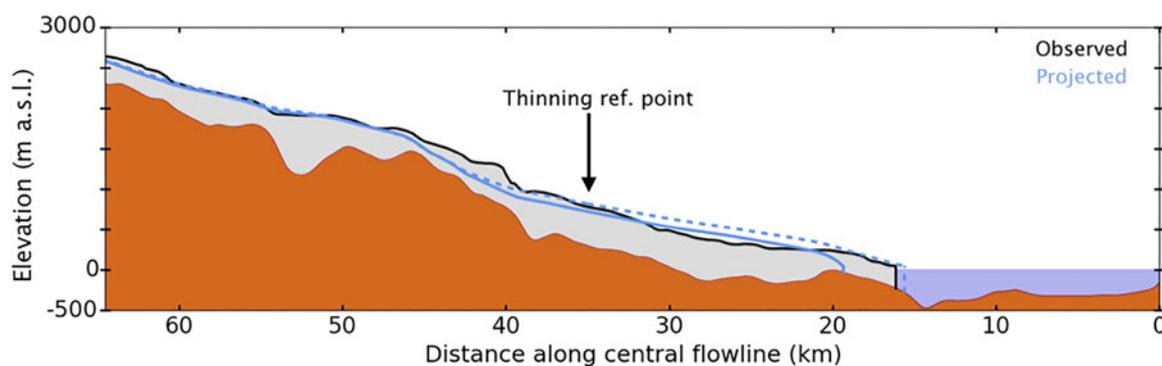
**Fig. 6.** Comparison of constant yield and effective-pressure yield criteria in simulating 2007 retreat from prescribing observed amount of thinning (210 m) at reference point (35 km upstream, black arrow). The centerline profile from 2007 observation (McNabb and others, 2012) appears with black outline and grey fill. Profiles projected using  $\tau_y = 150$  kPa and  $\tau_y = 130$  kPa +  $\mu(\rho_i g H - \rho_w g D)$  are solid and dashed blue curves, respectively.
