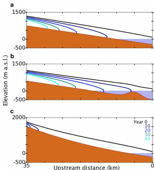
**Fig. 2.** Retreat of a perfectly plastic glacier under  $5 \text{ m a}^{-1}$  constant upstream thinning. Colored curves show initial profile (black) and profiles (blue scale) after 10, 20, 30 and 40 a of thinning. The idealized bed cases (after Oerlemans, 2008) shown are: (a) constant seaward-sloping bed, (b) seaward-sloping bed with overdeepening and submerged sill and (c) concave bed.
