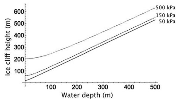
**Fig. 1.** Height of ice cliffs at the terminus produced by the model for yield strengths  $\tau_y = 50$  kPa (solid), 150 kPa (dashed), and 500 kPa (dotted) and water depths  $0 \text{ m} \leq D \leq 500 \text{ m}$ .
